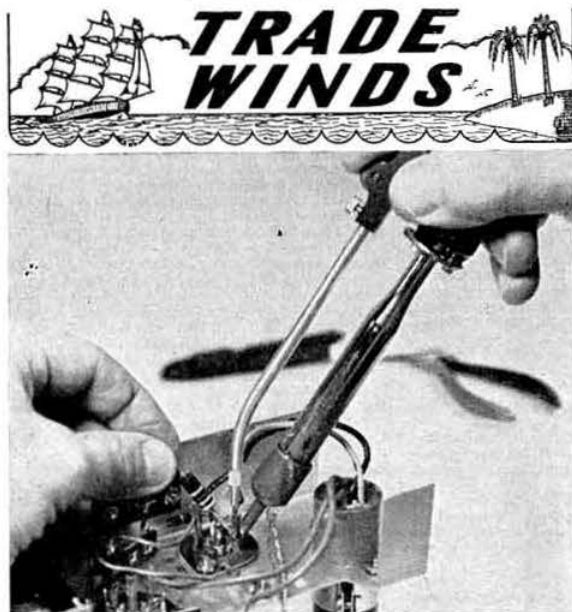
The "Third Hand" solder dispenser being used to attach a resistor to a valveholder tag. The soldering iron shown is an American model, but no trouble should be found in using the "Third Hand" with British types.
